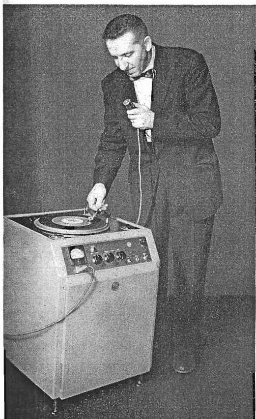
FIG. 9. Magnetic discs are easily recorded. The convenient microphone jack is just below the meter on the BA-51A Record/Reproduce Amplifier.
